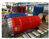
The technical principle of the transport and storage casks is the following: The radiation emitted by the radioactive inventory is safely
