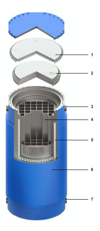
CASTOR® geo is the latest cask system by GNS. Based on well-proven components and state-of-the-art processes this system easily meets the individual requirements of customers worldwide for storage and transport of both PWR- and BWR-fuel assemblies.
