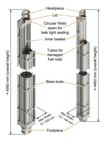
Quiver for casks for Pressurized Water Reactors
