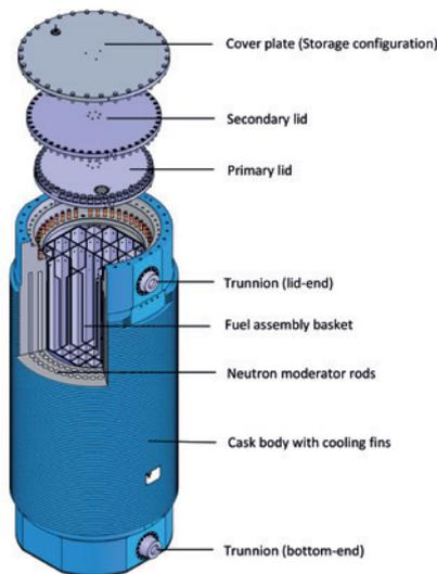
Fig. 3. Design Features of the CASTOR® V/52 (Storage configuration).
