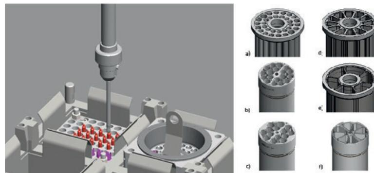
Fig. 4. Damaged fuel rods and handling tubes with fuel rod sections are placed in a receptacle, which is positioned in the fuel assembly storage rack. Next to that the quiver is waiting for the loading (left). Different internal baskets for varying kinds of bent damaged fuel rods (right).
