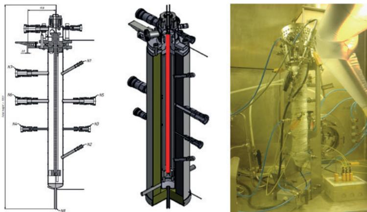
**Fig. 9.** Hot-cell installation for wetting and drying experiments on spent nuclear fuel segments: Design drawing of the two vessels: a large bottom vessel and a much smaller top vessel (left). 3D cutout view of the equipment with schematic indication of a mounted spent fuel segment (center). View of the equipment installed in hot-cell (right).
