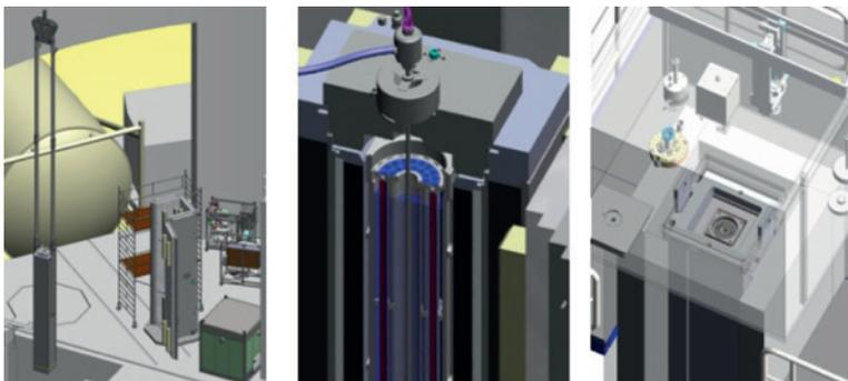
**Fig. 7.** The quiver inside the primary shielding is lifted out of the pool and into the handling station on the reactor floor (left). Dewatering of the quiver inside the handling station (center). View into the mobile hot cell on top of the handling station (right).
