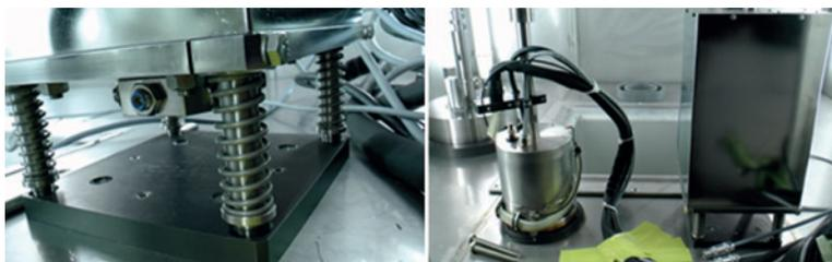
**Fig. 18.** Close-up of the lid screwing device (left), welding machine and lid screwing device (right).
