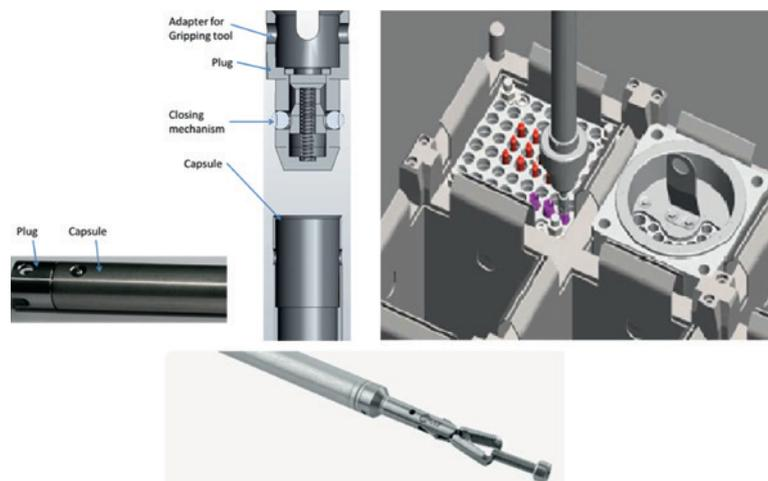
Fig. 5. Handling tube for the collection of heavily damaged fuel rods, smaller sections of fuel rods or even broken pieces down to the size of pellets (left). In analogy to the loading of fuel rods with an intact upper pin, the handling tubes are placed in the internal basket of the quiver (right). Example for a gripper to collect fuel debris for placement in cartridges before loading into the quiver (bottom).
