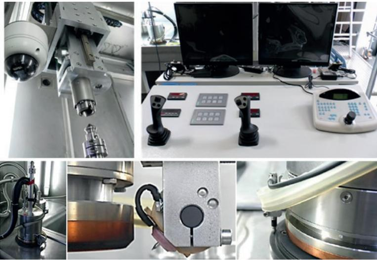
**Fig. 8.** The remote controlled handling device inside the mobile hot cell with one of the six cameras inside the cell (top, left). The remote control terminal which is placed next to the handling station (top, right). The remote controlled automatic welding device (bottom).
