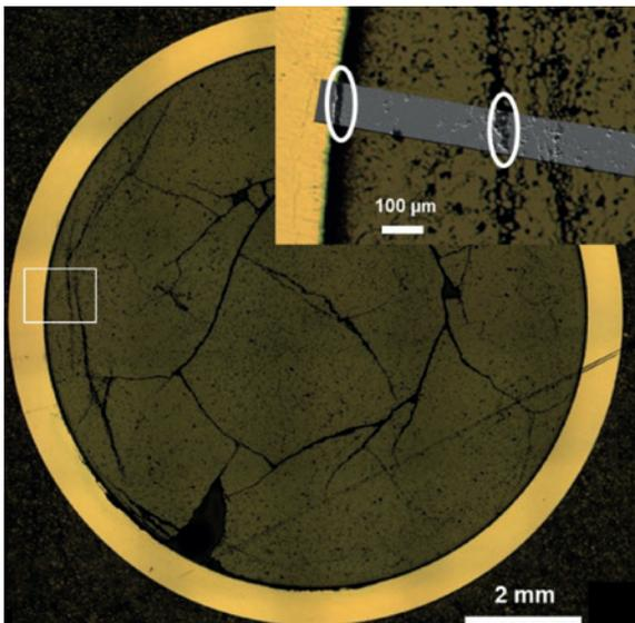
**Fig. 10.** Cross section of the spent fuel segment WET1, taken from the failed fuel. The cracks and gap do not show any particular severe degradation. The missing part on the bottom side is caused by sample preparation. Inset: detail of the gap region, with an overlay of a Scanning Electron Microscopy (SEM) image. The greater depth of view of the SEM allows one to better assess the width of irregular areas such as cracks and the pellet-clad gap than observations made from optical micrographs.
