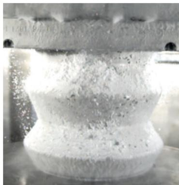
**Fig. 2.** Drop test at  $-40^{\circ}\text{C}$ , just before impact.
