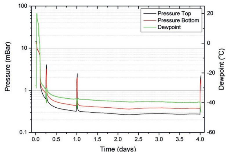
**Fig. 11.** Drying sequence with monitoring of pressure evolution in both top and bottom vessel and evolution of the pressure during a 30 minutes dryness test, performed after approximately 6 h of drying, 24 h and 96 h.
