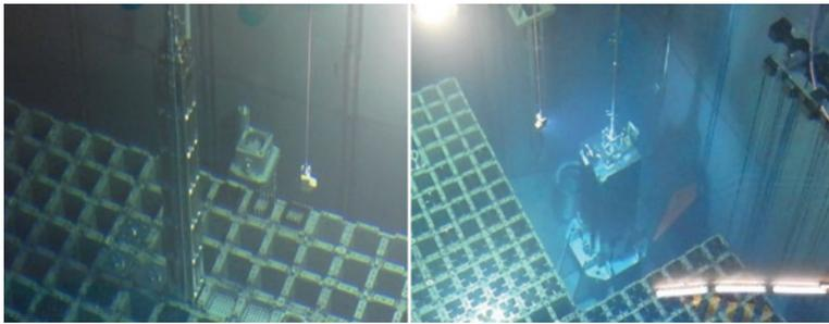
**Fig. 16.** Storage rack and quiver (left), top shielding on shielding basket (right).
