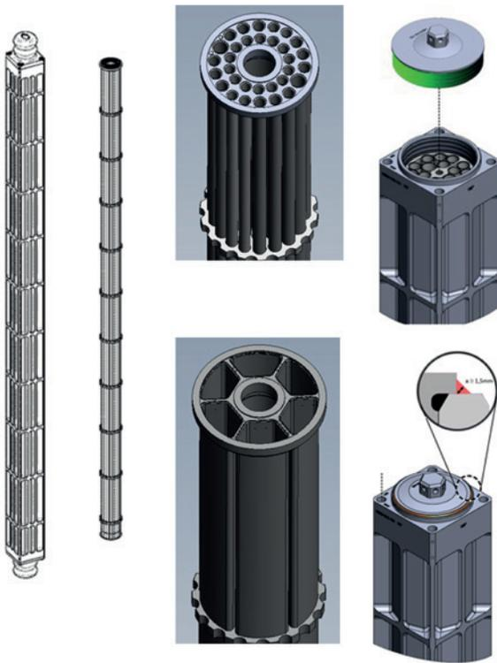
**Fig. 1.** PWR-quiver with head- and foot-piece, inner basket, 32AR (upper-) and 6AR (lower picture), lid of BWR-quiver (upper-), welded lid (lower picture) – (from left to right).
